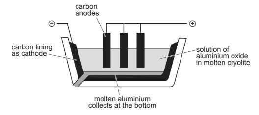
Which equation represents a reaction taking place at the anode?
